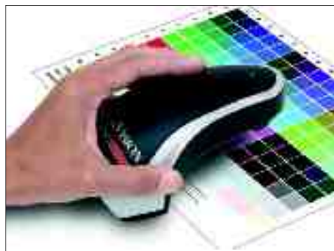
Creating a colour profile for your printer is easy. Simply run the spectroradiometer over the swatches provided
